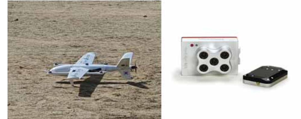
Shape of unmanned aerial vehicle and multispectral sensor
